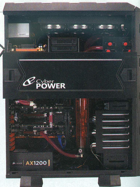
An Azza Fusion 4000 enclosure accommodates a gaming system below and a more modest WHS box up top.
